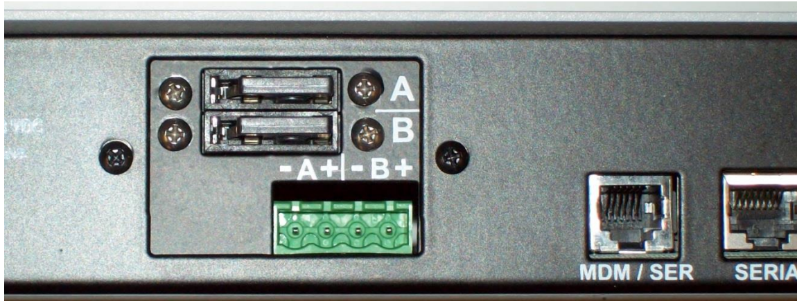
Figure 21 Close up of optional Dual Power entry showing fuses and polarity
